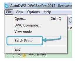
Option2. Hold "Ctrl" and click the drawings that you need one by one in current folder, when finished, right click on any of the highlighted file and select "Batch Print"
