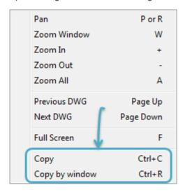
Option3. Hold "Ctrl" and press "C" to copy the current view or hold "Ctrl" and press "R" to copy a certain part of the drawing in clipboard.
